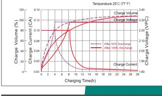
Charge Characteristic Curve For Standby Use
