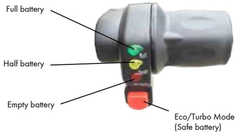
The red button located on your throttle is your Eco/Turbo Mode Button. When this button is pushed in your scooter will be in Eco Mode and your scooter's power charge. When the button is pushed out your scooter will be in Turbo Mode. While in this mode your scooter's speed and power is greatly increase. However you will lose distance per charge while in this mode.
