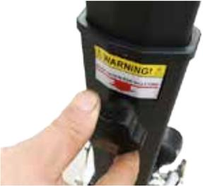
Turn the screw as below pictures to adjust the height of the handle pipe, do not unscrews it more than 3 turns.
