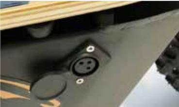
Lead-acid batteries can be connected to the charging socket of the scooter!
