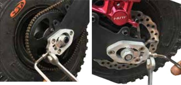
When the chain getting loosen, use the tools to adjust below chain tensioner to adjust it.
